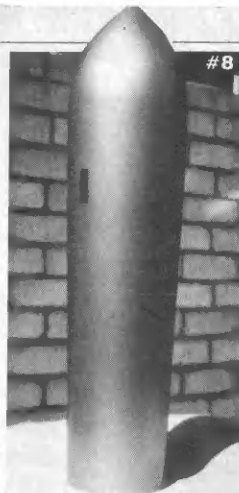
Below: The plaster tower mold on the shaper stand. The template had been released. Note the wooden bobbin end stops. The method of transferring the design drawing to the template is the same as described for the XM model.
